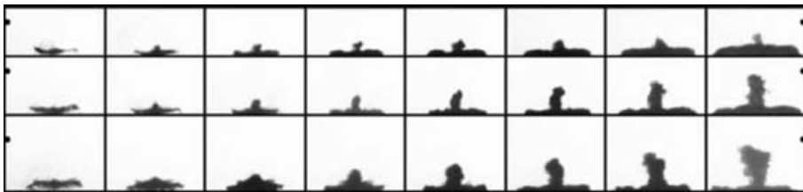
FIGURE 16. Onset of the counterjet for \gamma = 2.6, 2.2 and 1.8 (top to bottom), 10, 120, 250, 500, 1000, 2000, 4000 and 8000 ns after shock wave emission. R_m = 1.5 mm, frame width 0.97 mm. Note that the rigid boundary is below. The marks on the left-hand side of the figure indicate the horizontal position of the bubble creation location (reproduced with permission from Lindau & Lauterborn 2003).
